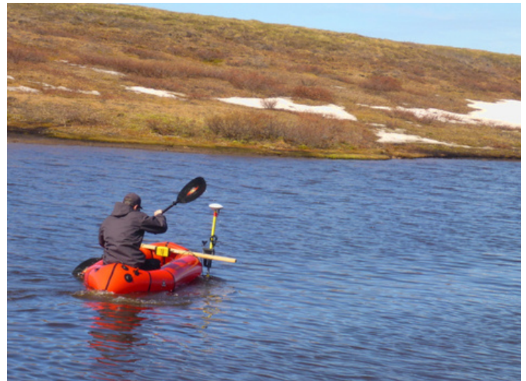
To supplement our drone data, Reyce Bogardus (now a PhD student with the University of Alaska Fairbanks' Arctic Coastal Geoscience lab) paddles an inflatable pack raft rigged with our sonar and GNSS equipment to collect 3D bathymetric data of a research lake.
